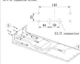
7. Tighten the screws No. 5, connect two hoses to  $G_{\frac{1}{2}}$ connector No. 6 and guaratee no leakage. Cut the end of PTFE taped connector by cutting machine if need to make connector shorter and repeat installation from step 4.
