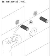
5. Unscrew the seven M4 screws with Allen Key, Slip out the wall cover No. 2 and then put out the Backcover No. 3.
